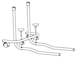
2. Use the two long handscrews to secure the 'C' shaped section to the two shaped 'L' sections.
