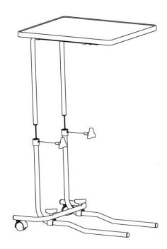
3. Connect the two sections of the table together as shown above. Adjust the table top to the required height and angle, then secure by screwing the 2 short handscrews clockwise in to the 'L' sections.
