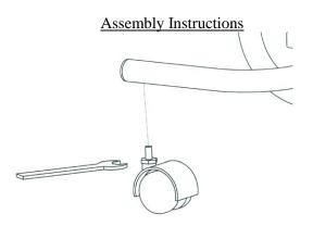
1. If required, attach any loose castors to the frame using a 13mm spanner (as shown in above diagram)
