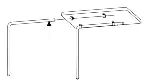
Insert the two chrome legs in the brackets located underneath the table top. Press the push button (arrowed) on the leg until slid through both of the brackets.
